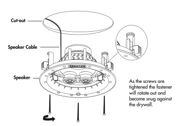
Center the speaker in the cutout. Rotate the frame as needed before tightening the screws. Tighten the screws equally until the clamps secure the frame. **Do not overtighten.**
